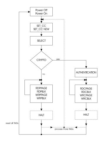
POWER OFF ... The read/write device turns off the 125 kHz transmitter to put the transponder in its initial (reset) state
