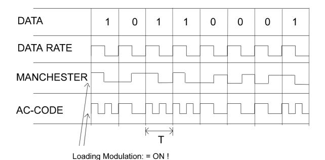
The first bit of the transmitted data always starts with the Modulator ON (loaded) state.
