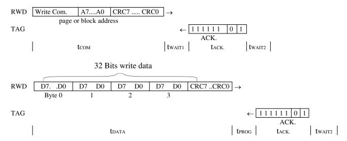
With a Write Page command the last part of this protocol is executed only once. With a Write Block command this part is executed one to four times, depending on whether the address indicates the beginning of a block or the beginning of one of the three remaining pages within that block.
