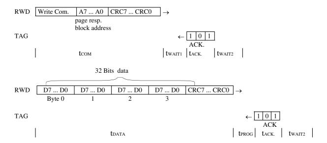
With a Write Page command the last part of this protocol is executed only once. With a Write Block command this part is executed one to four times, depending on whether the address indicates the beginning of a block or the beginning of one of the three remaining pages within that block.
