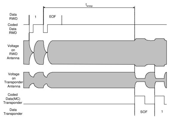
When receiving a End of Frame (EOF) condition from the Read/Write Device, the transponder waits  $t_{\text{wresp}}$  before transmitting data.
