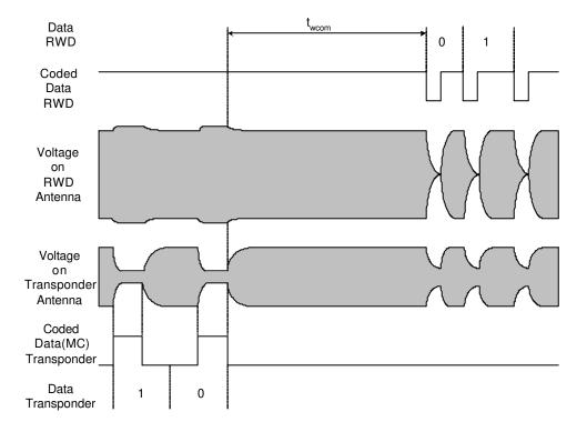
When the Read/Write Device has received the response from the HITAG S Transponder to a previous command, the RWD has to wait a time  $t_{\text{wcom}}$  before sending a subsequent command or Write data after a Write command.
