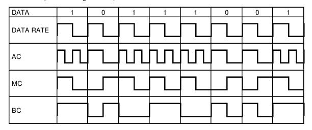
A high level of the above coding signals means the physical state 'modulator on' (field loaded), a low level means 'modulator off' (field unloaded).
