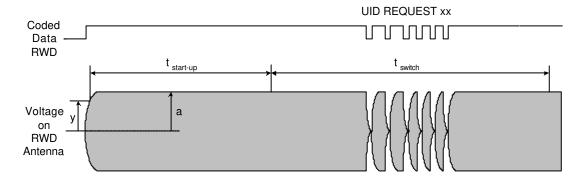
Within the time  $t_{\text{switch}}$  a HITAG S Transponder configured in TTF Mode can be switched into RTF Mode by a UID REQUEST xx command. The HITAG S Transponder responds to this command with the UID and changes into Init State .
