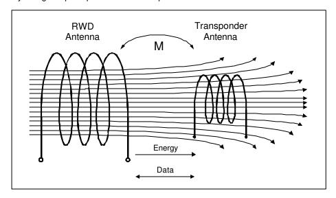
The RWD antenna generates a magnetic field. Some of the generated magnetic flux flows through the transponder antenna and induces a voltage there. The voltage drives a current and the transponder will start operating. As this current will be very small when the transponder is far away from the antenna, the HITAG S Transponder IC is designed for low power consumption.
