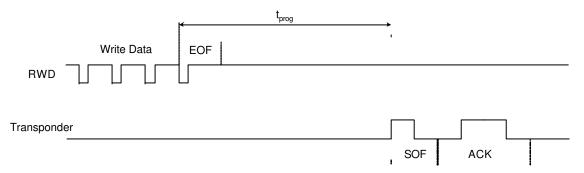
When receiving the EOF of the write data from the Read/Write Device, the transponder waits  $t_{prog}$  before transmitting the SOF and acknowledge to confirm correct programming.
