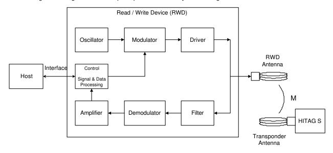
A control and data processing unit controls the modulation of the carrier signal and processes data coming back from the demodulator circuit.
