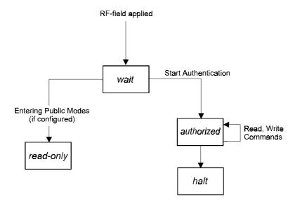
After entering the RF-field the transponder waits for a command to start the authentication.
