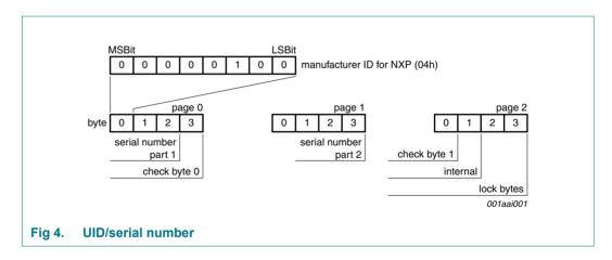
According to ISO/IEC14443-3 BCC0 is defined as CT  $\oplus$  SN0  $\oplus$  SN1  $\oplus$  SN2. Abbreviations CT stays for Cascade Tag byte (88h) and BCC1 is defined as SN3  $\oplus$  SN4  $\oplus$  SN5  $\oplus$  SN6.
